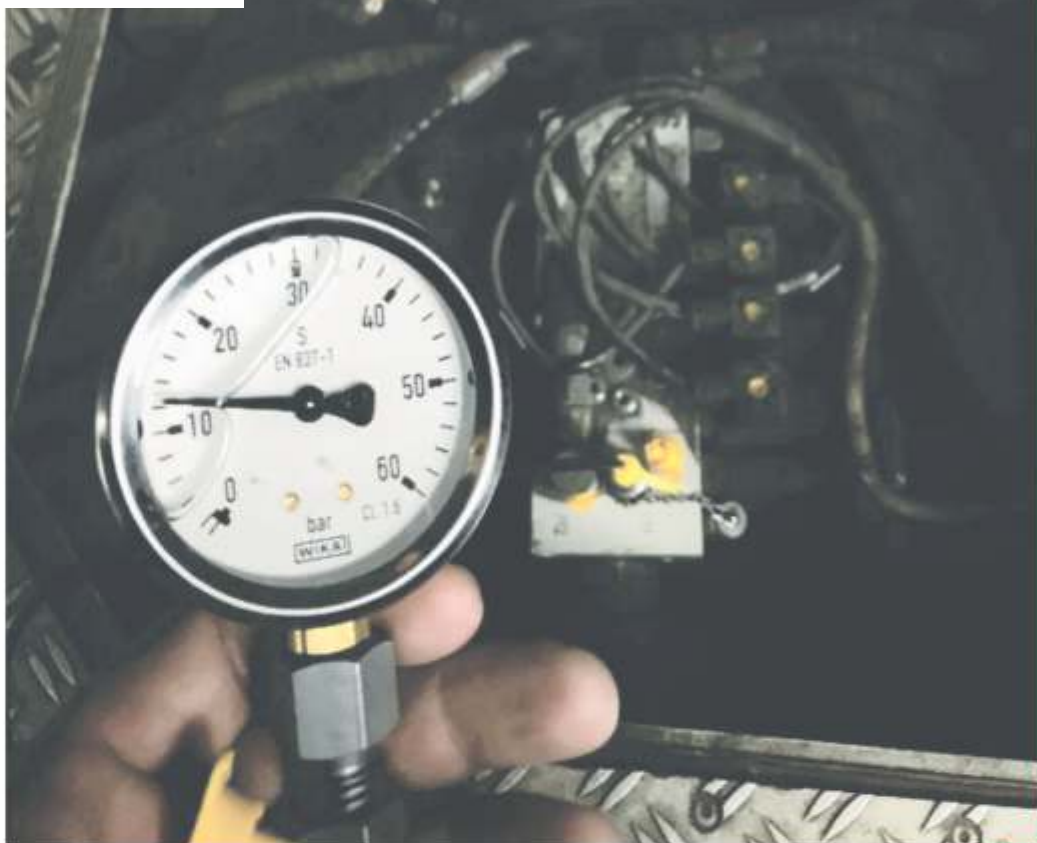
Drop in operating pressure in the hydraulic system to 12 bar was quickly recovered to the correct level of 20.7 bar by a service pump.
