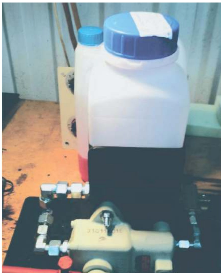
ATG's hydraulic pump for maintaining the right oil level in the articulation hydraulic system.
