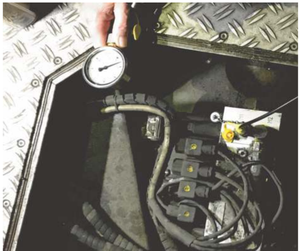
Pressure measurements using a manometer in the hydraulic control block.
