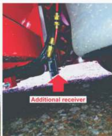
An additional receiver with a central control unit is connected by electric wire harness supplying power and information about the tire pressure and temperature in the CAN format.
