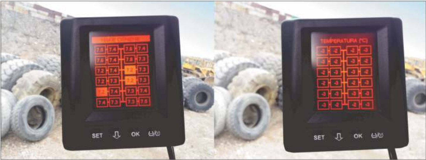
Pressure and temperature are controlled in the tires of the two rear axles of the tractor unit and four axles of the semitrailer - in total in 24 wheels.
