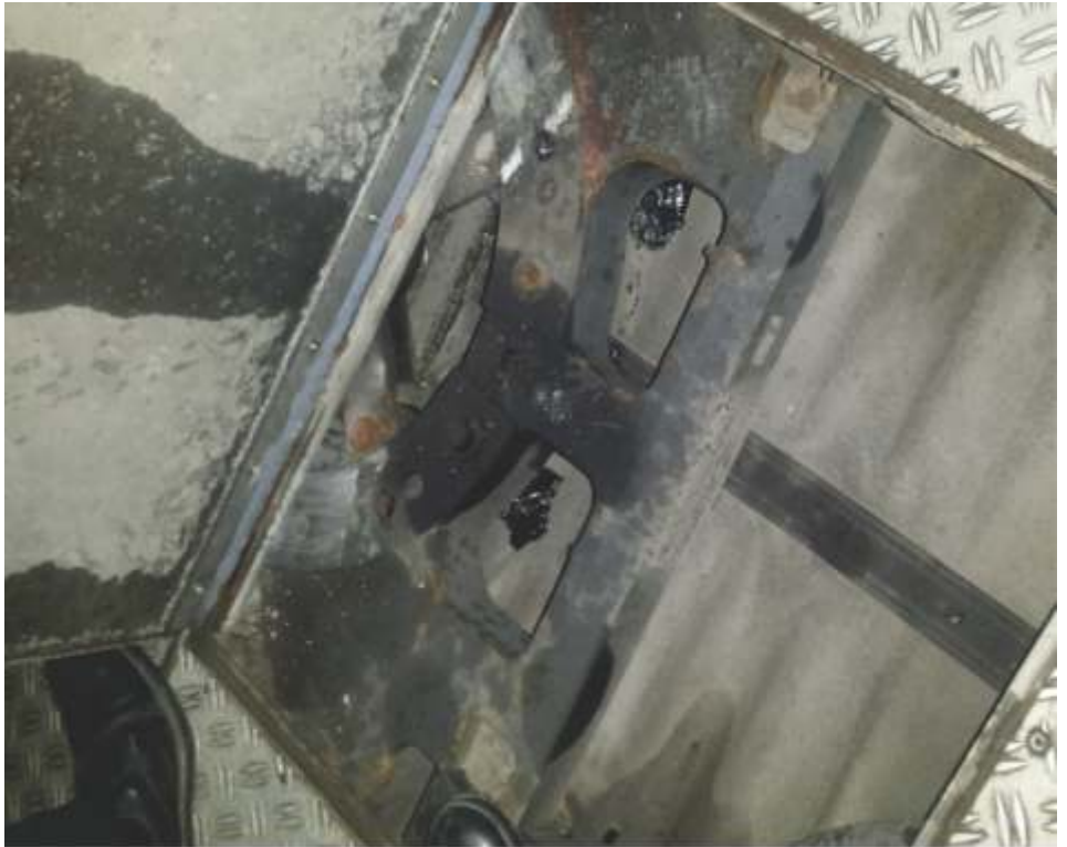
Access to a turntable area of the articulated system from the level of the internal service flaps.
