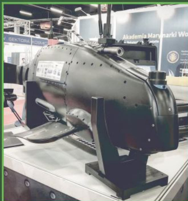
BB-2590 SMBus battery was used in a propriety biomimetic underwater robot called "Cyber Fish", which has been constructed by engineers from the Cracow University of Technology for the Polish Naval Academy.
