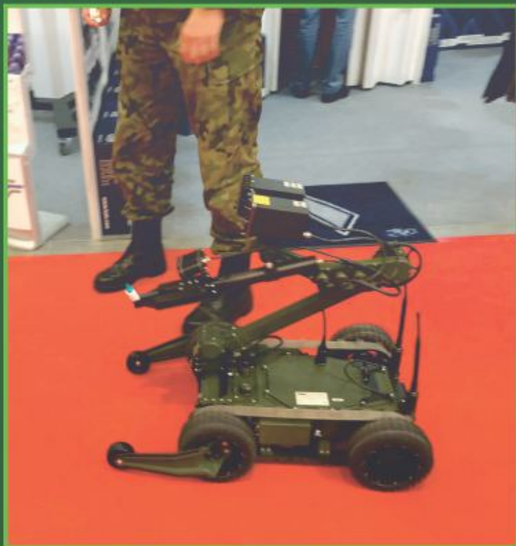
„Balsa” Light Reconnaissance Robot constructed by Warsaw PIAP with lithium-ion BB2590 SMBus Denchi battery.
