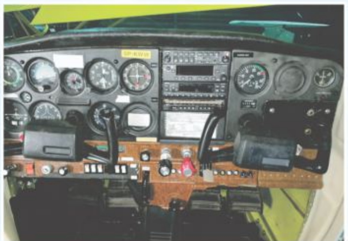
New equipment of Cessna 152 – above - GMA 342 audio panel and GTR 225A radio.
