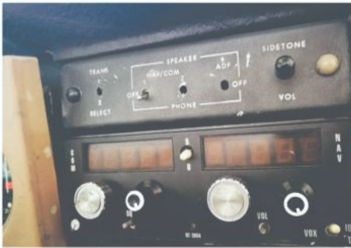
One of the aero club's aircrafts before modification – with original Cessna equipment – audio selector and RT 385 radio.
