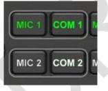
There are two pushbuttons associated with the transmitter selection. The two left buttons (MIC 1 & MIC 2) control which transceiver is selected for transmit. The right column of pushbuttons (COM 1 & COM 2) allows selection of the receiver audio. Push the MIC button to select the desired transmitter.
