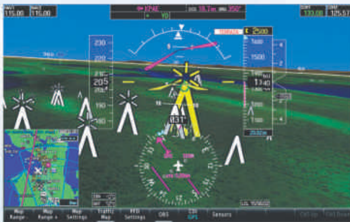
3D imaging of mast-obstacles by the SVT system on the Garmin G1000 PFD screen.
