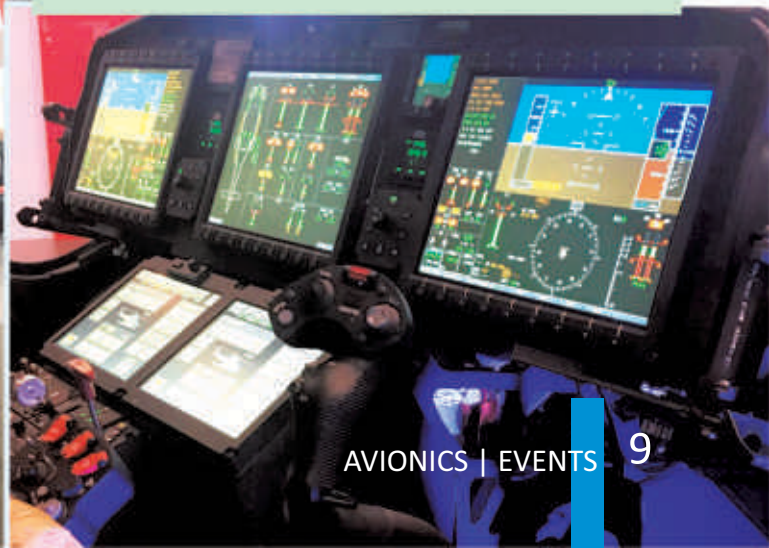
AW 169 helicopter, manufactured by Finmeccanica-AgustaWestland with participation of PZL-Świdnik, equipped with Collins Aerospace avionics system.
