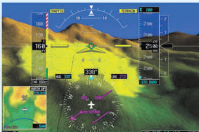
Imaging of mountainous terrain by Garmin's Synthetic Vision Technology (SVT).
