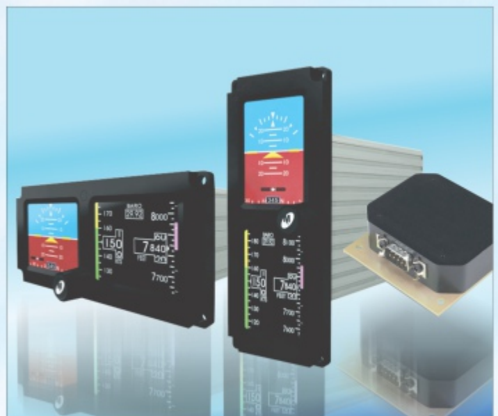
Standby Attitude Module (SAM) from Mid-Continent Instruments and Avionics is available in horizontal and vertical orientation. In both versions with MD32 Magnetometer included.
