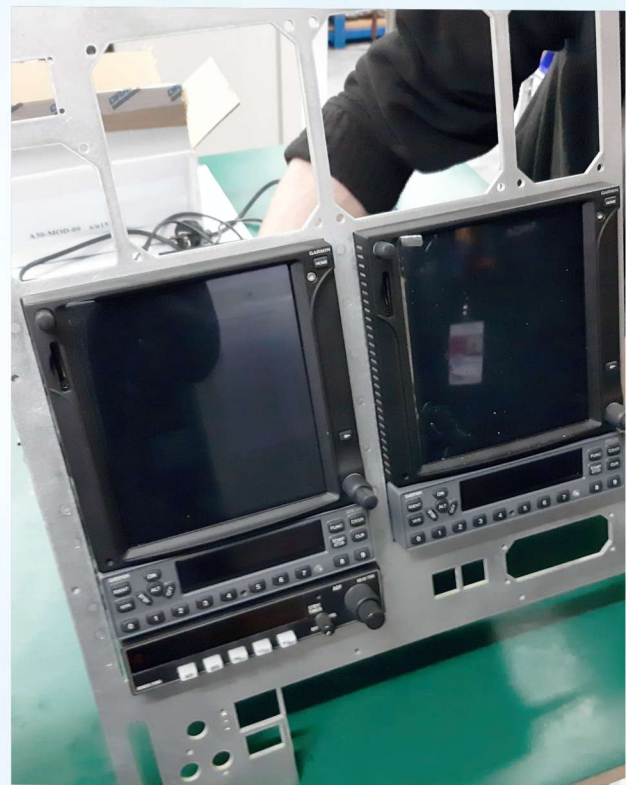
The finished instrument panel with new GTN 750 touchscreen navigators before powder painting.
