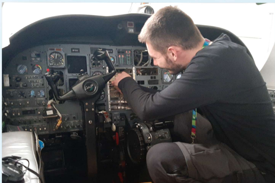
The removal of current avionic equipment.
